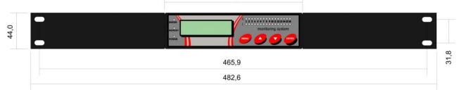
Mechanical drawing of ATM-06D data logger (without cables and connectors):
