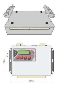
• data logger ATM-06D is fixed<sup>2)</sup> by means of the holder on DIN rail at low current switchboard - <u>working position is with input connectors downward</u>
