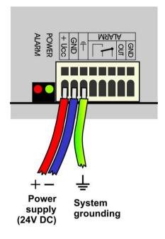
If system is not grounded properly, it is a danger of state, when system floats on variable potential against all other circuitry. It can cause communication dropouts, occasional resets and in extreme case damage of some peripherals. Especially when using pulse power sources (e.g. PS-ATM) it is strongly recommended to ground the system.
