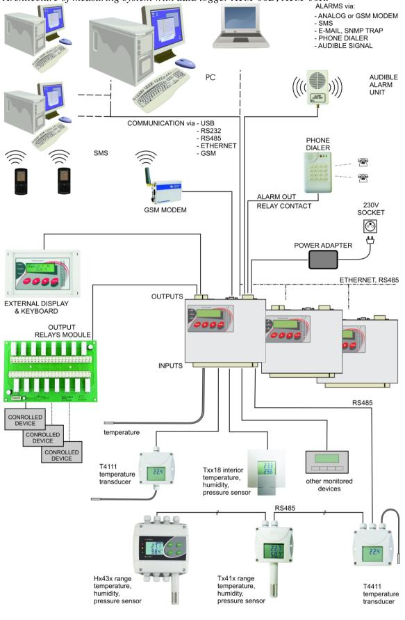
Architecture of measuring system with data logger ATM-06D, ATM-06R:
