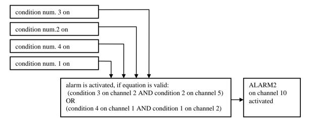
Alarm is active, if input conditions are valid. By means of combination of conditions you can solve also complex situations including remote control. Some actions last during all alarm time (audible indication, ALARM OUT output activity, visual indication, relay closing), other actions last only at the moment of alarm creation (SMS message, e-mails).
