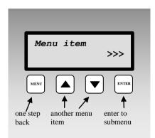
Press MENU key in basic display to enter the data logger Menu. Use  $\blacktriangle$ ,  $\triangledown$  keys to go through all menu items. Press MENU key to leave menu to the basic display.
