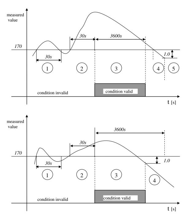
To renew validity of condition measured value first must drop below specified limit and then to exceed the limit.
