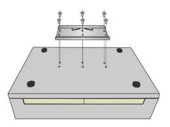
• data logger ATM-06R is mounted to 19" rack<sup>1</sup>
