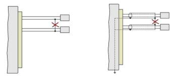
• **do not create hidden earth loops** - do not connect cable shielding at end device side, if these device do not have terminal designed for shielding. Shielding must not be connected to outer metal parts of the device nor with other devices. Do not use shielding as a signal lead.
