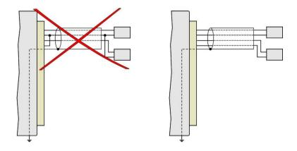
• It is recommended to earth data logger at one point – there is a special terminal on power terminal. This earthing will work correctly, if system would not be grounded at other point at the same time.
