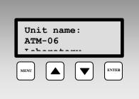
Display after connection power to data logger.
