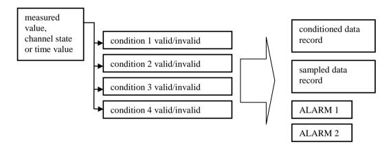
Data logger enables to set condition depending on measured value, on time and condition, which validity is remotely controlled. Each from four conditions it is possible to switch on for evaluation. Binary inputs has lower number of possibilities to set conditions, setting is analogical.
